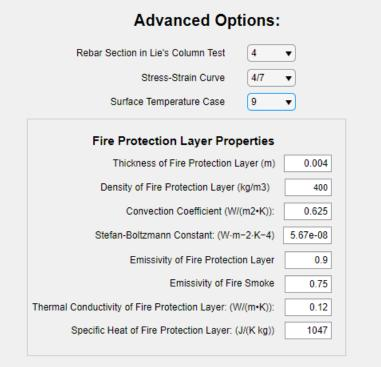
If 4/7 is selected in Stress-Strain Curve, program takes 4 for compact and 7 for non-compact and slender sections.
