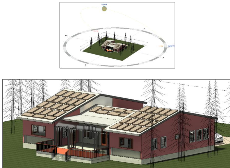
Figure 8. Revit model shown with shadows on June 21. Note that the overhangs prevent the solar gain from penetrating through the direct gain windows as well as the sunspace and Trombe wall.
